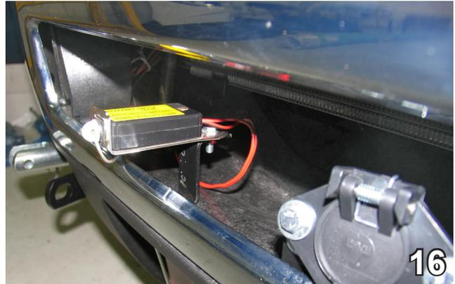
15. Reinstall the bumper. Install the electrical bracket, using 1/4-20 x 3/4" hex bolts with 1/4" flat washers and 1/4-20 whiz nuts.
