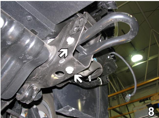
8. Using the 18MM socket, remove the two metric bolts from the side and bottom of the tow hook. Pull the tow hook forward. Do this to both sides of the vehicle. **The tow hooks will not be reinstalled.**
